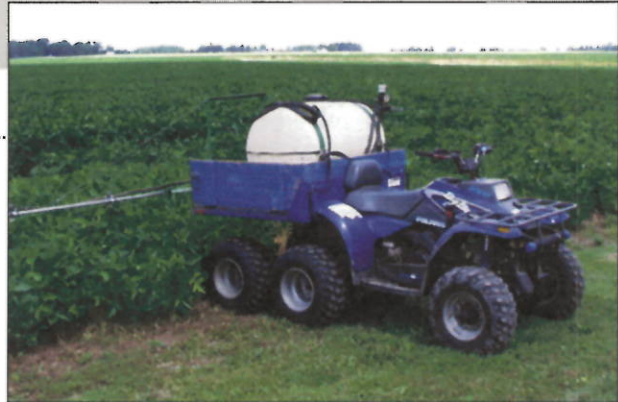
Figure 7. David Eshelman uses a 6-wheeler to spray small weed patches. This applicator is equipped with its own spray boom and hand wand for spraying weeds in the field or along fence rows.
