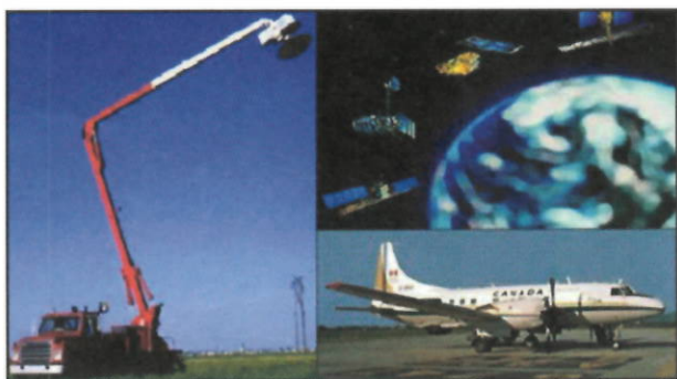
Figure 2. Sensor Platforms: Left, ground measurements; right top, satellites with an variety of sensors; right bottom, aircraft with sensors at bottom of plane.
