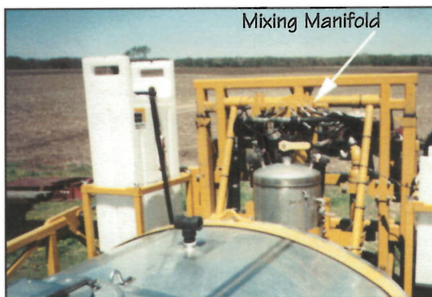
Figure 3. Site-specific herbicide applicators often carry only water in their bulk tank, such as the 1000 gallon tank on this sprayer. The concentrated herbicide is then pumped into a mixing manifold where it is diluted with the water to achieve the proper rate before entering the spray boom. (photo provided by Aventis CropSciences)
