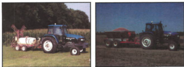
Figure 2. Most of the VRT equipment can be transferred between different applicators. For example, a global positioning system used during a pesticide application may also be used during the fertilizer application.
